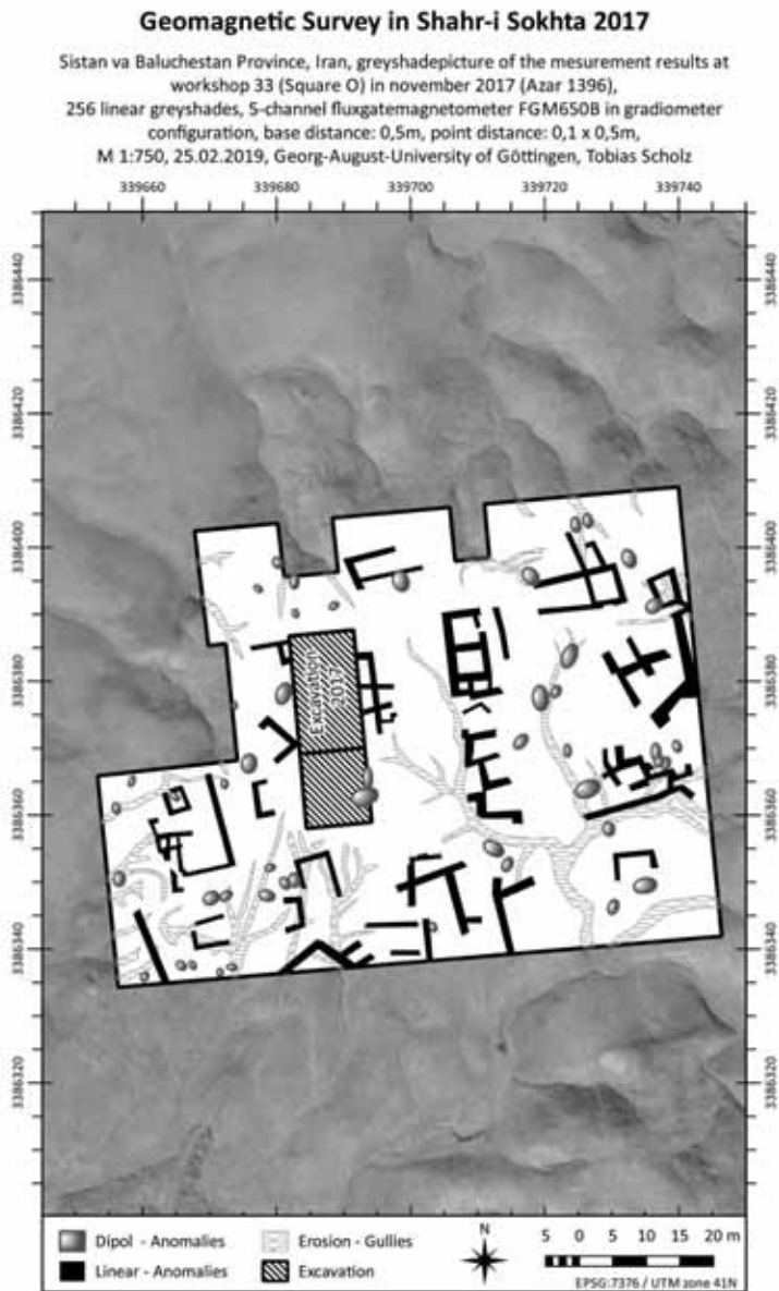
Fig. 8: preliminary results of geomagnetic survey in Area 33 at Shahr-i Sokhta.
